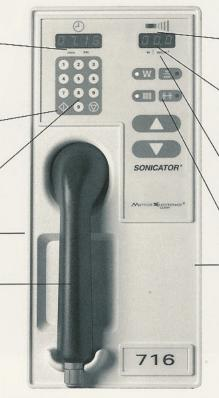
Patient Contact Indicator signals warning if inadequate coupling occurs.
